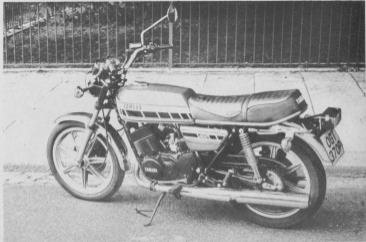
Good-looking. The 350-ib lightweight RD400 has (we think) clean, functional styling, with individualistic touches like all-black finish for engine and crankcase
