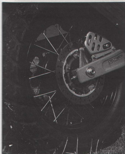
The rear brake is quite powerful, but it lacks feel and locks up easily
