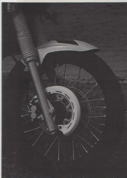
The front brakes should be excellent, but they lack power and feel very squidgy
