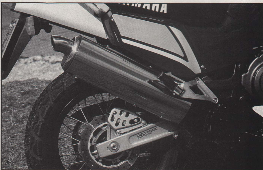
The silencer is really hideous, but the Deltabox swingarm ensures a good ride at the back
