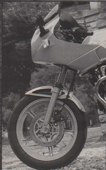
Twin 270mm discs are effective, and still part of Guzzi's linked system
