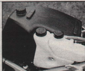
All three tanks fill up under petrol tank cover
