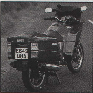
Panniers are a decent size and don't appear to leak. Note the built-in leg protectors
