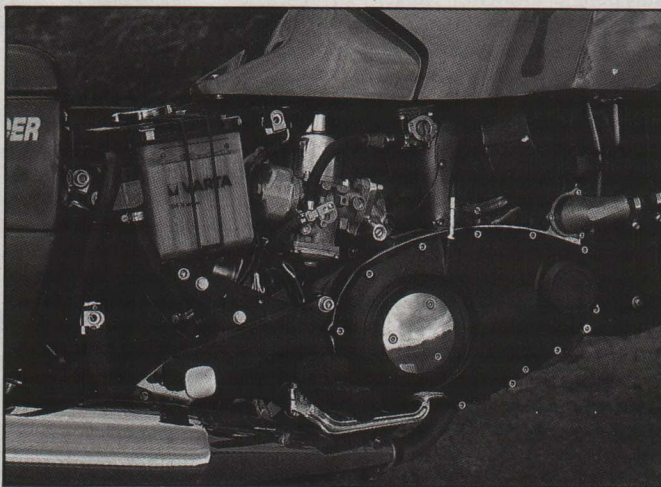
Water-cooled rotary engine has masses of grunt and is ultra-smooth
