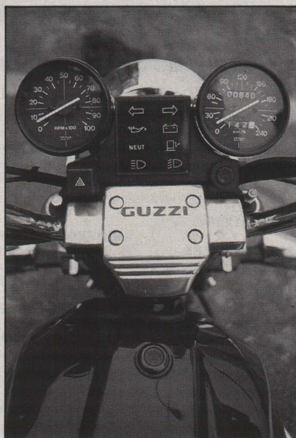
Fascia shows Guzzi's commitment to progress, warning lights are comprehensive and highly visible, hazard flasher switch sits conveniently to port.
