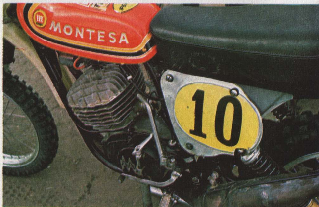
Capra VR benefits from Montesa's race testing; the works bike shown here has the latest cantilever rear suspension.
