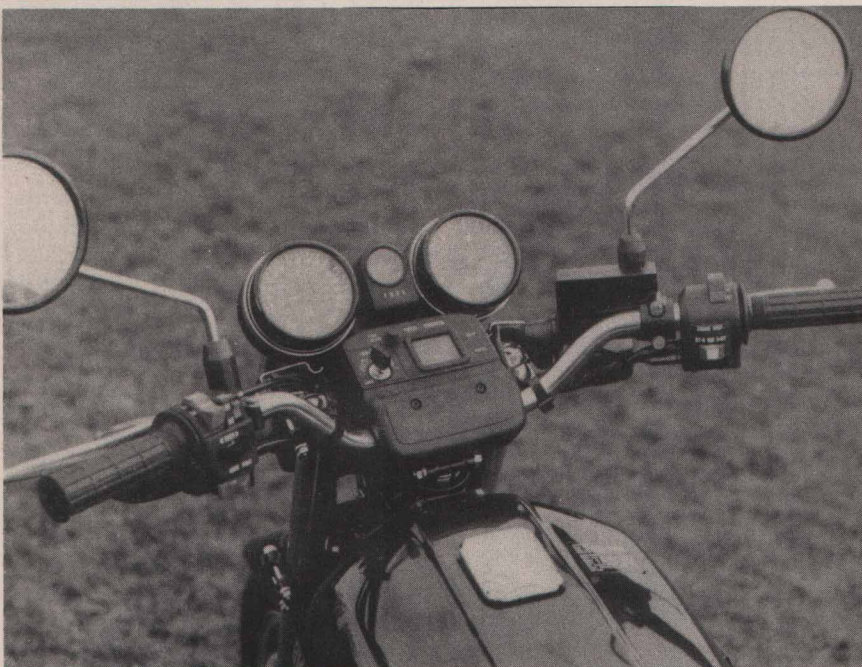
Electronic instruments and large but fumbly switchgear
