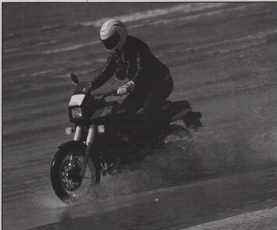
Off-road handling is compromised by too much weight on the front wheel, too little suspension travel
