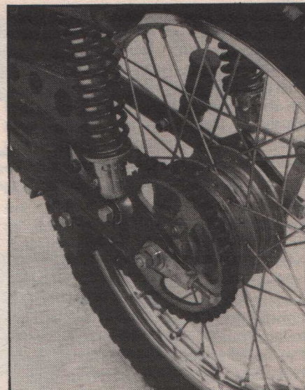
Chain guard hardly lives up to its name! No chain tensioner is fitted, but guide is fairly substantial.
