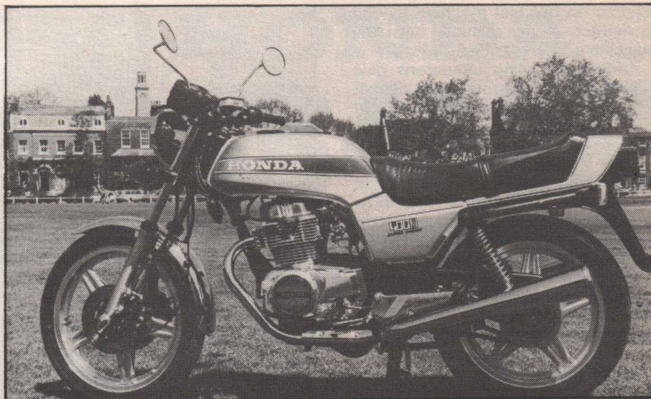
Comstar wheels now feature all alloy construction. Handling is first class although machine is far from being a lightweight: tyres performed well in wet or dry.
