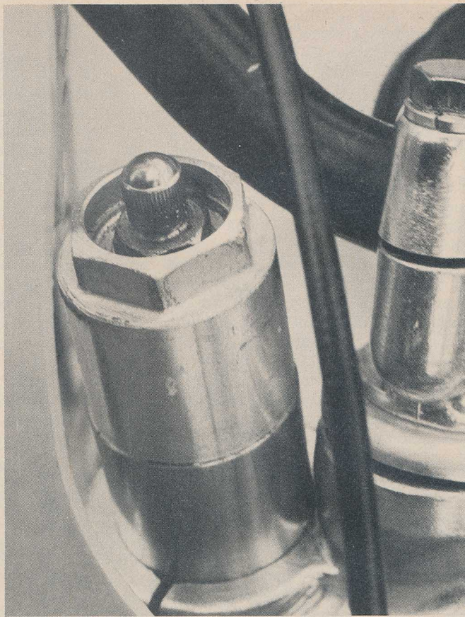
Air valve is slightly recessed in extended caps. Combination of longer tubes and cap allow for larger volume for air spring adjustments.
