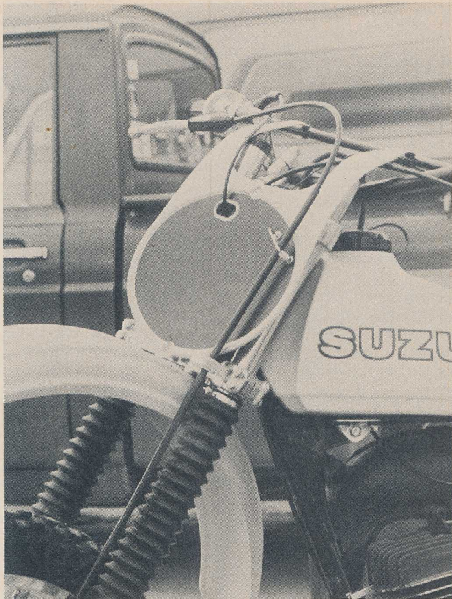
Double flap number plate and improved cable guides and stays reduce chances of cable snagging. Plate is fastened directly to triple clamps.
