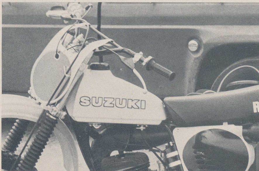
Tank filler hole is large and handy. Plastic tank will take a lot of abuse—decals won't.
