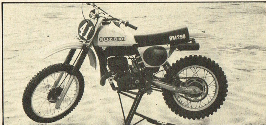
Dirt Werkes stand effectively lifts both wheels off the ground for maintenance. It has good stability in the dirt and works great in the garage.
