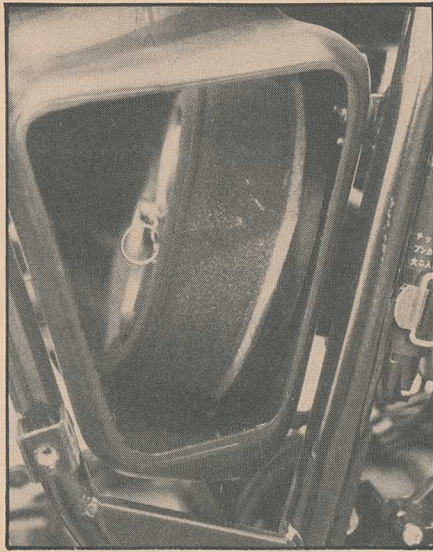
Air box design and execution is good. Filter changes are made easy by "trap door" at side of box. Number plate side cover seals access hole with foam sealing strips.
