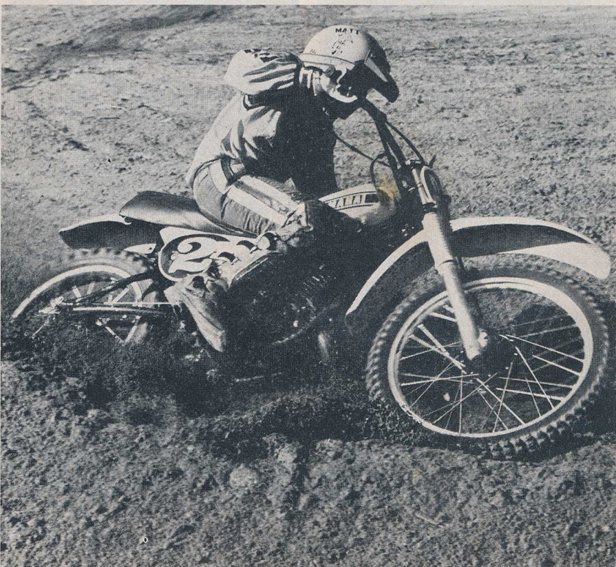
Superb forks with leading axles. They felt stiff for lighter riders at first, but under actual racing conditions, they proved to be about ideal.
