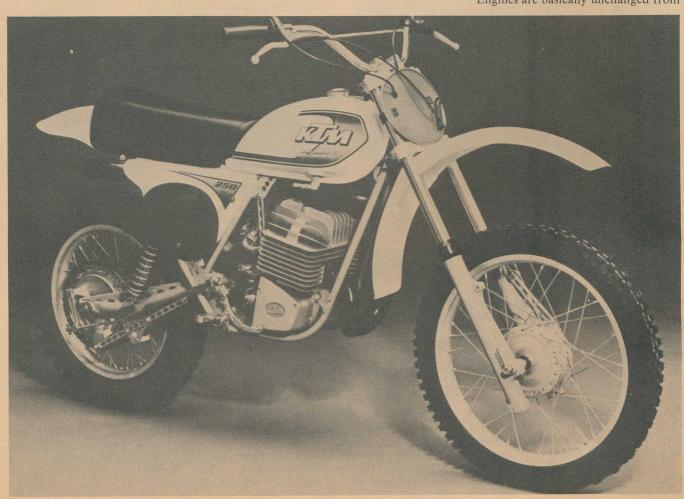
the past models. Massively finned piston-port barrels are Bing-fed and sparked by Motoplat capacitive discharge ignitions. Cases and sidecovers are pressure die cast magnesium.
