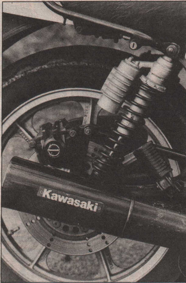
Showa remote reservoir rear units give a firm ride and could be contributing to the rather vague, wallowy handling.
