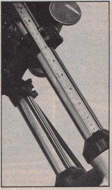
Extended fork measures seven inches from top of wiper to the bottom of triple clamp. Forks slide up 1½ inches with weight of bike when using S&W's SP1820-18 fork spring. (They sell for \$13.95 a pair.) A superbly smooth ride is obtainable.
