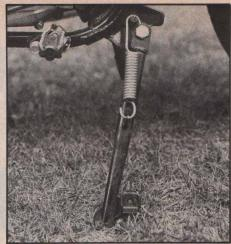
We shortened the side stand one inch, but we should have made it 1½ inches because the bike is lower than we thought. The stock shift lever and footrests were left "as is;" this is not too low because the XL is pretty narrow, making it difficult to drag anything.
