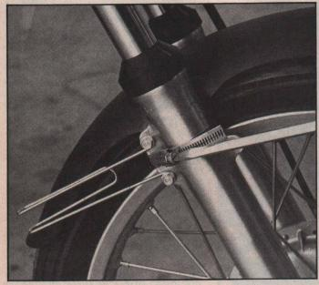
Funny Fender can be purchased in either white or black, for \$15. You will have to do some trimming around fork legs in order to slide the fender close to the tire. Normal hose clamps are used to hold it on and we found wrapping clamps around the fork boss works best.
