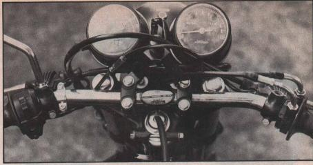
These are Harley-Davidson drag bars from MCM, measuring about 24 inches from end to end. Left side is a squeeze, especially since a compression release has been fitted. Routing of control cables is simply a case of common sense. Bend them as few times as possible and don't kink them. Front brake cable loops very high and throttle cables go from the top. The new set-up allows a normal seating position; you don't lean on the bars.
