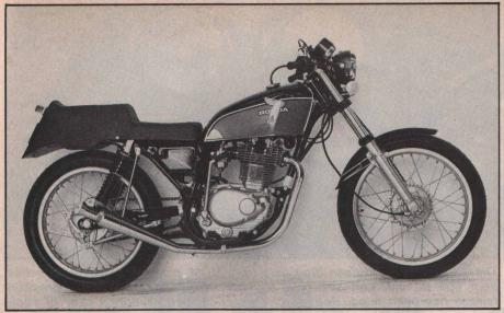
"Working model" has had white plastic fender and seat gray-primed for photographic reasons. The front wheel uses 19-inch DID alloy rim fitted with 3.25 x 19 Avon GP tire; rear is a 4.10 H x 18 Avon GP. MCM's down-pipe saves almost 15 pounds but it is not nearly as quiet as stocker. The lowered bike boasts a 28-inch seat height.
