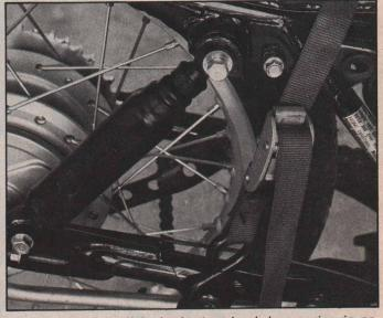
We mounted a 1½-inch shorter shock less spring in order to check out wheel clearance. The stock trials tire rubs upper frame brace. We used the S&W H525-2 gas bag shock (\$32.95 each) and the S1270-10 spring (\$8.33 each). Note clever use of the tie-down strap, finger-tight bolts. We had to cut about 3/32 of an inch from the shock bushes and eyes.
