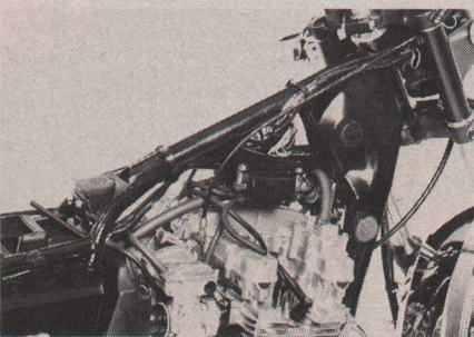
Hefty gusset plates add strength to the steering head area to reduce flex.
