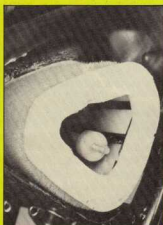
Above: Chain tensioners are new to all YZs. It's one of few tensioners we've seen that doesn't tear up the chain. Keep everything lubed and adjusted and you shouldn't have any problems. Right: Air filter arrangement hasn't changed; they're still using a pair of those fuzzy elements. They're harder to clean but do a good job of keeping water out.
