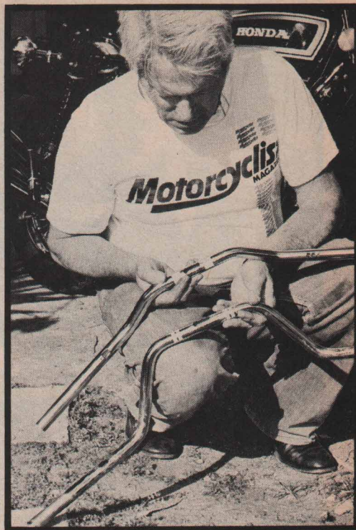
Of course I did the hard part, cutting holes in these undiscovered Honda tri-cycle bars for wires, etc. These bars come plain, without any wiring holes.
