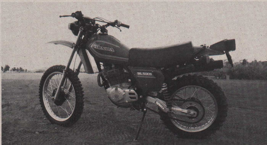
The Work's Shocks will be supplied with triple-rate springs—they do a good job of effectively soaking-up the small bumps and handling the XL's enormous weight too.
