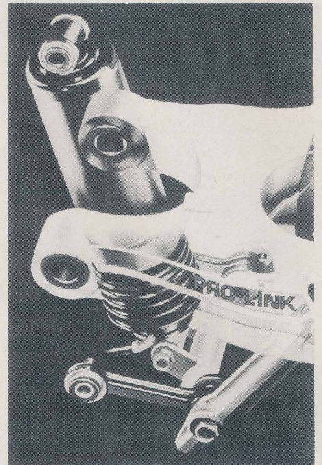
Pro-Link suspension's rising rate action gives excellent rear wheel control. Air-assisted coil is easily adjusted.
