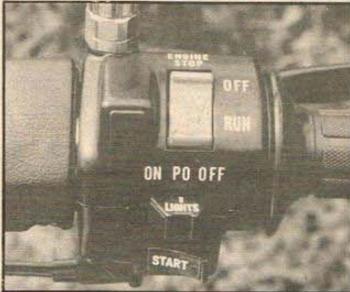
Controls for the right and left hands. Despite the busy appearance of the left-hand control module, above, everything falls naturally to the thumb without confusion
