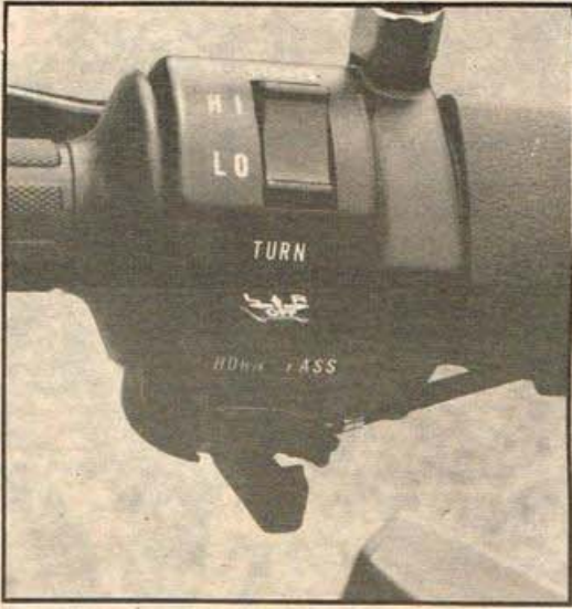
Controls for the right and left hands. Despite the busy appearance of the left-hand control module, above, everything falls naturally to the thumb without confusion
