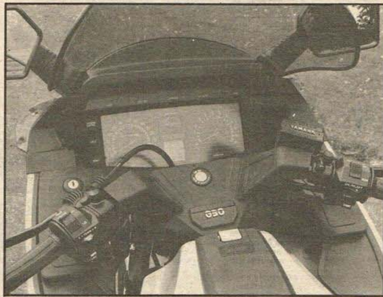
Comprehensive and compact cockpit (but no clock!) with the central ignition switch/lock amid the moulded plastic handlebar shield. Air-assisted forks are interlinked to attain balanced and more convenient setting.
