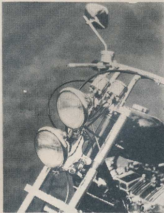
ABOVE: Twin Bates headlamp shells hold halogen bulbs.
