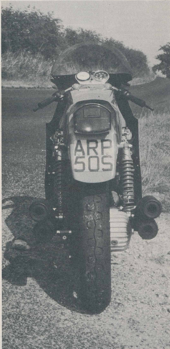
Rear end of the MV Magni Monza is dominated by Magni's curvaceous and very musical pipes. John Lee retained the standard shaft drive set up rather than fit the Magni chain kit purely for convenience's sake.
