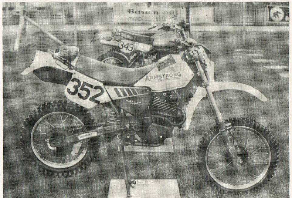
A very early arrival for scrutineering — and almost the only British machine in the event. The Armstrong's engine is the popular Rotax four-valver
