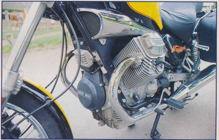
Carburettor-fed, Digiplex-ignition engine develops 48bhp
