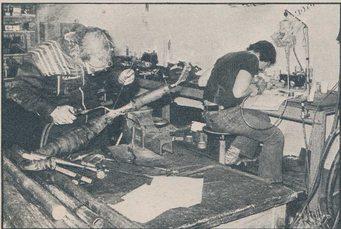
Out in the workshop Kel Carruthers gets down to the task of welding a damaged exhaust pipe. The race team have the use of the machine shop that is regularly used by normal staff.
