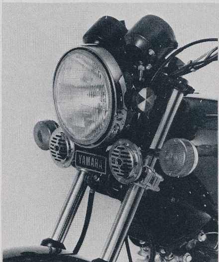
The huge eight-inch quartz headlight is plenty powerful, as are the dual horns.
