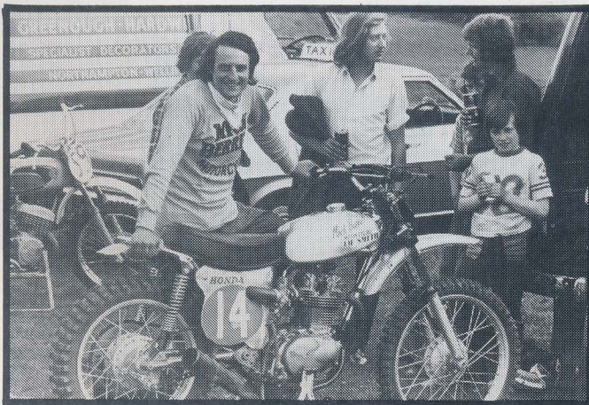
This XL250 in a Cheney 250 BSA frame was put together by Northampton dealer Mick Berrill for employee Sam Smith (pictured) to debut at Hawkstone Park in March 1973. Weight was pared to 231lb.
