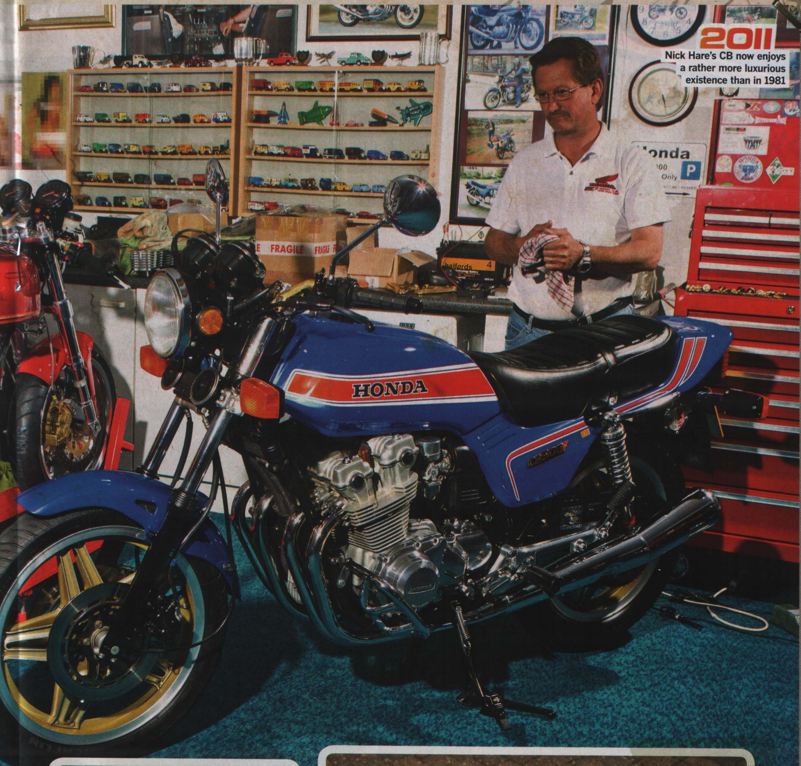
Honda FVQ shocks look the part but have a reputation for fading
