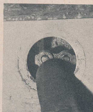
19 The chain tension can be inspected by lifting out the rubber bung. Check sitting on the bike
