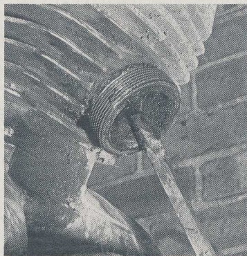
5 As long as you are careful not to touch the piston, you can scrape the carbon out of the exhaust port
