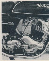
MODEL: Norton Commando 750 MCM ISSUE TESTED: August, 1968 TOP SPEED: 122mph SS¼ MILE: 12.8sec/104mph PRICE: £456.97 ENGINE: ohv four-stroke twin
