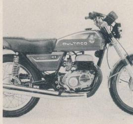
GEARBOX: five speed constant mesh CLUTCH: wet multiplate IGNITION: electronic LIGHTING: six volt battery and flywheel generator FUEL CAPACITY: 2.86gal WEIGHT: 243lb (dry)
