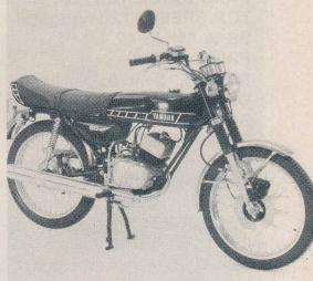
GEARBOX: four speed constant mesh CLUTCH: wet multiplate IGNITION: magneto LIGHTING: 6 volt battery and alternator FUEL CAPACITY: 1.4gal WEIGHT: 159lb WHEELBASE: 45.7in FRONT BRAKE: single disc REAR BRAKE: single leading shoe drum FRONT WHEEL: 2.25 × 17 REAR WHEEL: single leading shoe drum
