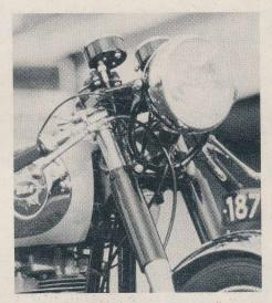
MODEL: BSA Gold Star B34 MCM ISSUE TESTED: not tested TOP SPEED: 115mph (estimated) SS1/4 MILE: 14.5sec (estimated) PRICE: £260.40 (1955) ENGINE: ohv single cylinder four-stroke DISPLACEMENT: 499cc BORE X STROKE: 85 X 88mm COMPRESSION: 8.0 POWER: 40bhp at 7000rpm (claimed) TORQUE: 32lb-ft at 6000rpm (claimed) LUBRICATION: dry sump
