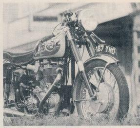
GEARBOX: four speed constant mesh CLUTCH: wet multiplate IGNITION: Lucas magneto LIGHTING: 6 volt battery 60 watt dynamo FUEL CAPACITY: 4gal WEIGHT: 416lb (dry) WHEELBASE: 56in FRONT BRAKE: 8in single leading shoe drum REAR BRAKE: 7in single leading shoe drum
