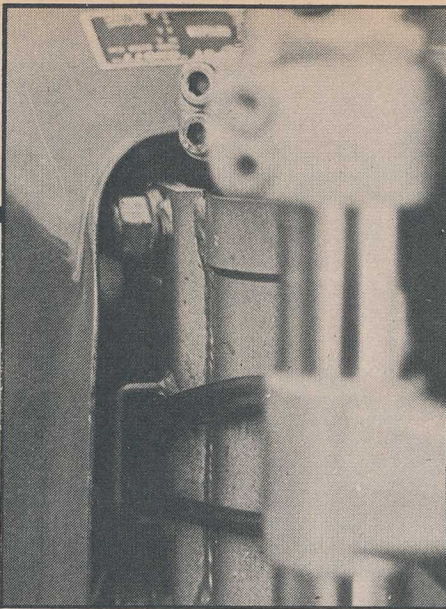
The Chott's bolt-up adjustable steering head allows a choice of three castor angles for on- and off-road riding.
