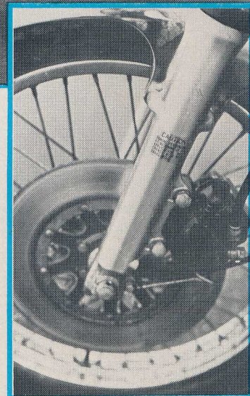
Warning sticker on the front forks reads like an apology for the brake's pathetic performance in the wet. When cold, the brake doesn't work at all.
