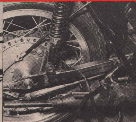
The Yamaha frame is standard, except for this swinging arm, built to extend the wheelbase and keep front wheel off the ground
