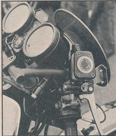
Home-made ace bars give the effect of clip-ons and are tailored to the rider.
