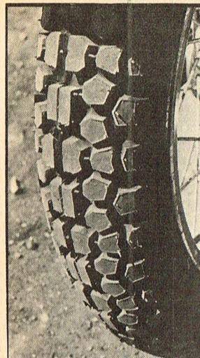
The block tread Barum S23 tyre performs well on and off the road.
