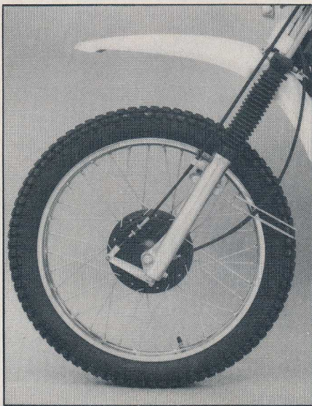
Long-travel, leading-axle forks spoilt by a lack of damping. Braking is one of the bike's best features, with lots of feel at the front and a fully-floating rear unit.
