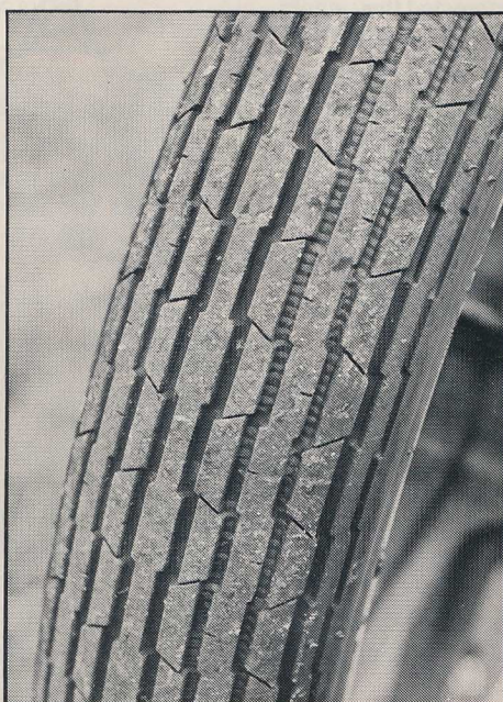
Wider sections are used on the GP model and both tyres are tubeless.
