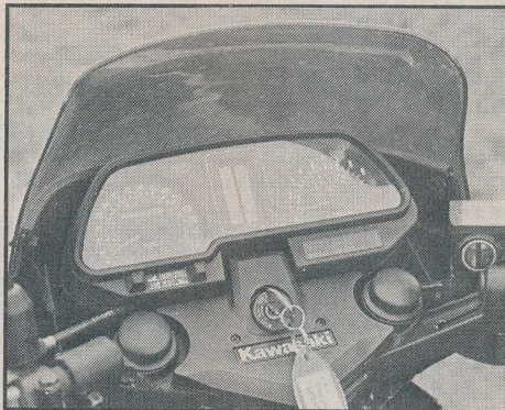
Instruments now include a voltmeter and LCD fuel gauge along with safety checks and tell-tale warning lights.
