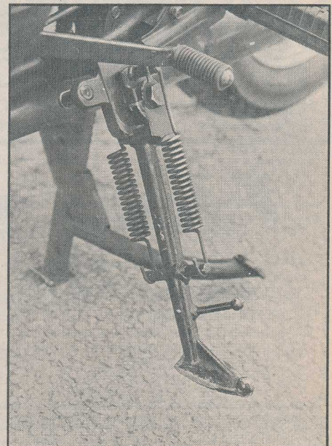
The high technology sidestand, along with its various cut-out switches, overrides and warning systems . . .
