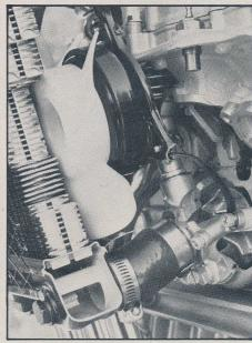
The black disc is a new-technology electric motor which drives the radiator fan. Its incredible thinness cuts the bike's wheelbase 2.8 inches.
