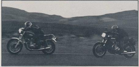
Surprisingly the Yamaha XS Eleven Special pulled the big Kawasaki in most throttle roll-ons, especially those beginning in third or fourth gear at midrange revs. Downshifting the Six gives it an edge over an unshifted Yamaha.
