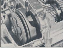
This is one of four shock absorbers between the crank and rear wheel to help control drivetrain snatch. Two are metal like this, two are rubber.
