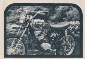
The Wombat has the edge in handling with its longer 52.5 in. wheelbase. It features a low 30.75 in. seat height, 14.75 in. crankshaft height and an ample 9.5 in. ground clearance for a lower center of gravity and better balance. You can adjust the rear shocks 6 ways to suit your weight and the terrain.
