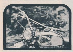
The Wombat's 2.8 gal. fuel tank features a large quick-fill cap to save precious seconds. The 70 degree quick throttle eliminates a "second handful" to reach full open.
