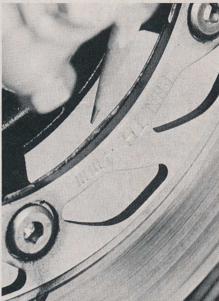
Honda damped vibration—and therefore brake squeal—with paper gaskets placed between the front disc carrier and the hub.
