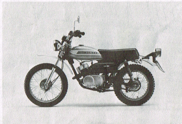
KM90 A midi-bike built like a big bike 1-cyl/2-stroke 99cc Rotary disc valve Primary kick 5-speed Dry weight 76kg/168lb
