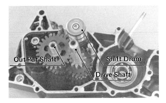
•Apply liquid gasket to the engine fitting surface of the left crankcase half, and fit the crankcase halves together using a press on the end of the crankshaft.
