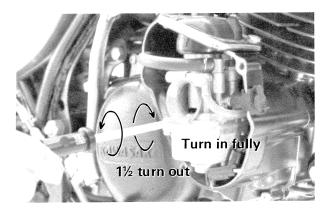
**NOTE:** Do not screw in the air screw forcefully; turn it just until it stops.
