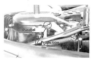
•Turn the clutch adjusting screw in to just where a resistance is felt, and then tighten the lock nut.
