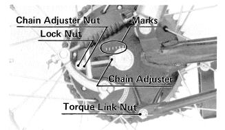
•With the chain adjusters, adjust the chain slack to  $15\sim 20$  mm ( $0.6\sim 0.8$  in.). Adjust so that the mark on the left chain adjuster comes to the same swing arm mark that the right chain adjuster mark comes to.
