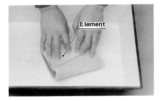
•Soak the element in a 10:1 gasoline/oil (SAE 30) mixture (10 parts of gasoline to 1 part of oil), and then, after it is dry, fit the element back in the air cleaner box properly so that no unfiltered air will enter the engine.
