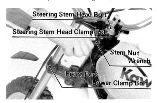
•Tighten the front fork lower clamp bolts (4).
