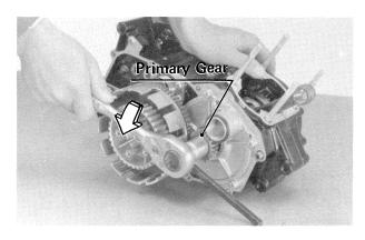
•Straighten the bent portion of the clutch hub washer, and remove the clutch hub nut (19 mm).
