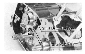
•Check to see that the crankshaft, driveshaft, and output shaft all turn freely.
