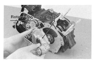
•Remove the rotary disc.
