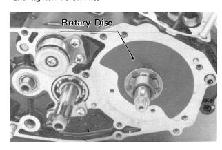
•Replace the thrust washer, output shaft idle gear, thrust washer, and then circlip back on the output shaft.
