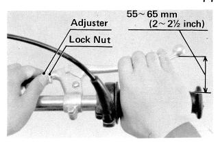
If the adjuster at the brake lever has reached its limit, adjust the cable with the adjuster on the lower end of the cable.
