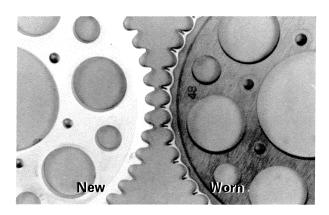
NOTE: Inspect the sprockets for wear, warp, and cracks.
