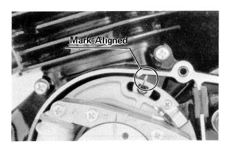
•If the marks are not aligned, loosen the lower magneto base screw, shift the position of the base so that the marks are aligned, and tighten both screws securely.
