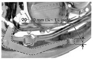
•Turn the adjuster at the rear of the brake cable to obtain the proper amount of play.
