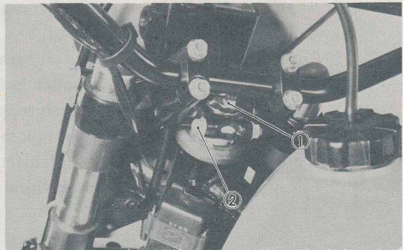
1. Steering fitting bolt 2. Stem pinch bolt
