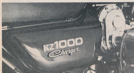
West drilled holes in the drive cover to eliminate mechanical noise harmonics. Otherwise kit is unchanged.
