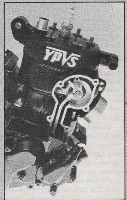
Power Valve's mechanical linkage Porting regulated by engine speed.
