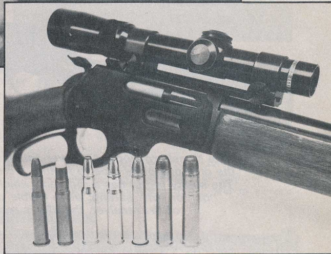
The Marlin Model 336 is available in a wide range of calibers, including (left to right): .30-30, .35 Rem., .307 Win., .356 Win., .375 Win., .444 Marlin and .45-70.
