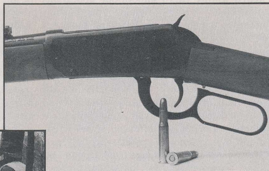
The traditional Winchester M-94 has a narrow, slab-sided receiver and an underbarrel tubular magazine.
