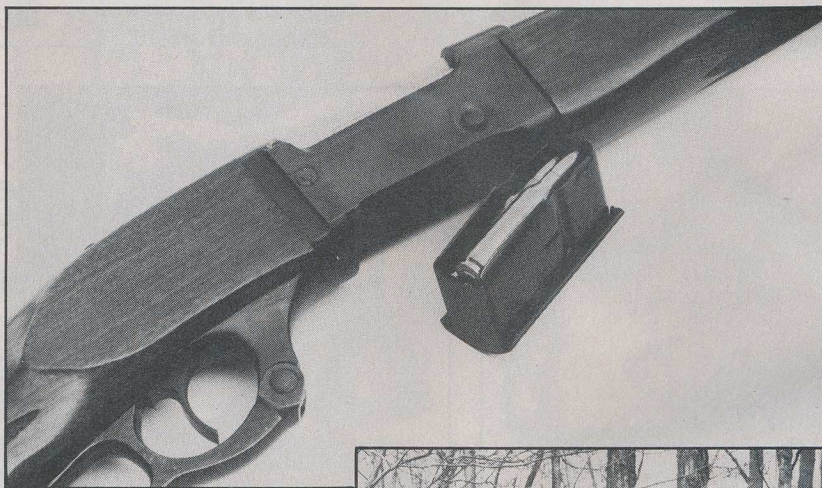
The Mossberg Model 479 lever-action rifle (above) is the only one of its type to feature a crossbolt safety. The safety (right) has a red band which indicates the "on" or "off" setting; when visible on the left side of the receiver, the rifle is ready to be fired.
