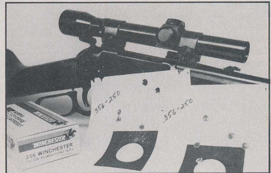
Winchester's new Angle Eject Model 94 makes possible the low mounting of a scope directly above the receiver, as empties are now tossed out the side instead of from the top. Impressive 2 1/2-inch, 100-yard groups (right) were fired using 250-gr. .356 Winchester ammo.
